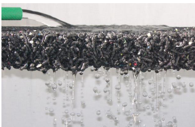
Figure 9-36 – Example permeable paving with piped outlet (Interpave)
